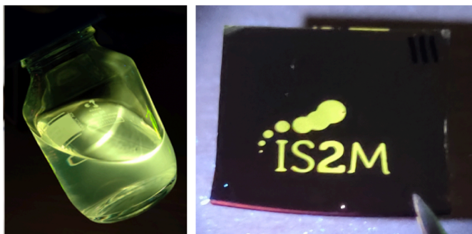
Figure : Photographs of the ZnO colloidal solution (left) and patterns on Si obtained by laser direct write Deep-UV photolithography (right) under UV-light illumination
